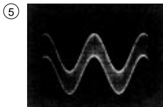
IC301 Pin 6 REC mode 2.2Vp-p
