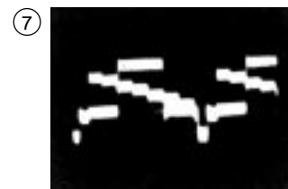
IC301 Pin 41 PB mode 400mVp-p
