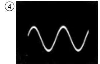
IC301 Pin 7 REC mode 1.4Vp-p
