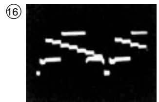
IC301 Pin 43 PB mode 400mVp-p
