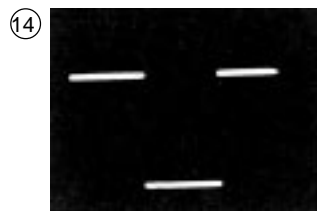
IC301 Pin 11 PB mode 3.2Vp-p
