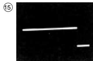
IC301 Pin 10 PB mode 1.8Vp-p
