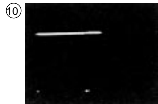
IC301 Pin 24 PB/REC mode 5Vp-p
